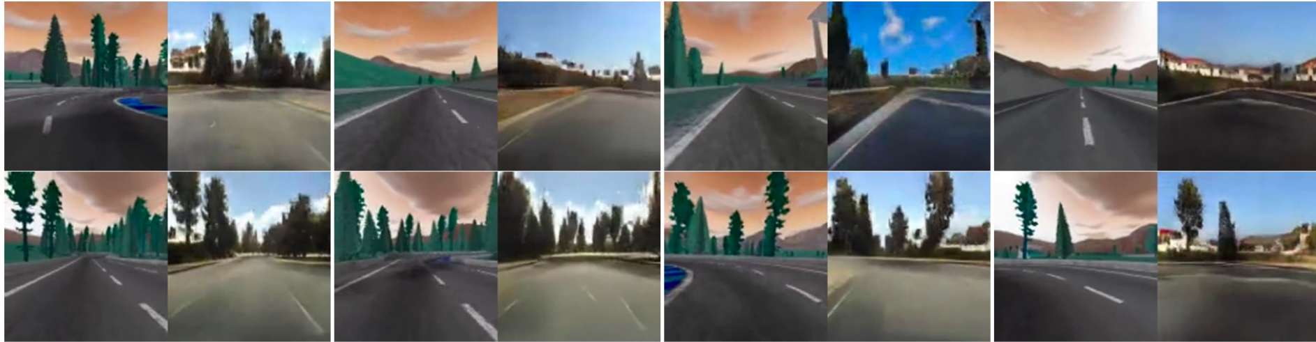
Figure 4: Examples of Virtual to Real Image Translation. Odd columns are virtual images captured from TORCS. Even columns are synthetic real world images corresponding to virtual images on the left.
