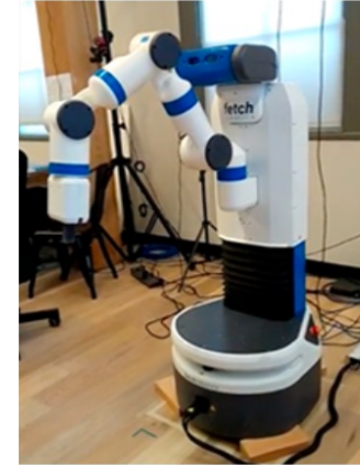
Fig. 2. Our experiments are conducted on a 7-DOF Fetch Robotics arm. Left: Real robot. Right: Simulated MuJoCo model.
